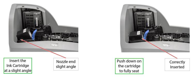
**Step 4:** Verify that the cartridge is properly installed. The cartridge should appear tilted at a slight angle when fully seated. Replace the 'Center Cover' by setting it back on the unit vertically.
